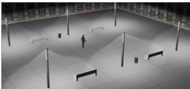
Eclairage symétrique circulaire (places, squares, jardins, parkings...) Circular symmetrical distribution (squares, parks, car parks...)
